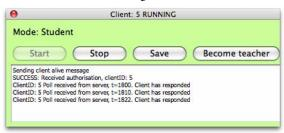
A green background means that the test client is running successfully. You can see a log of the communication the client has received from the server in the pane at the bottom of the test client window.
