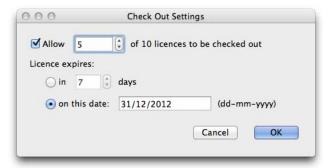
To enable check out licences, switch on the **Allow** *x* **of** *y* **licences to be checked out** checkbox. By default, the number of licenses to be checked out defaults to half of the total number of licences available, but you can change this to as many or as few of the available licences as you like.
